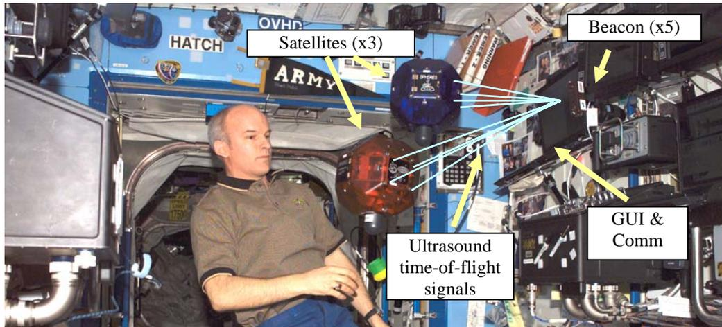
Figure 1 SPHERES hardware components operating aboard the ISS (Picture courtesy of NASA)
