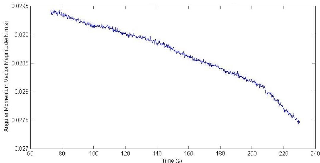
**Figure 4.2 TS16 P251 T2-3 Fluid Slosh: SPHERE Only, X Rotation - Total Angular Momentum for Drift Only**
