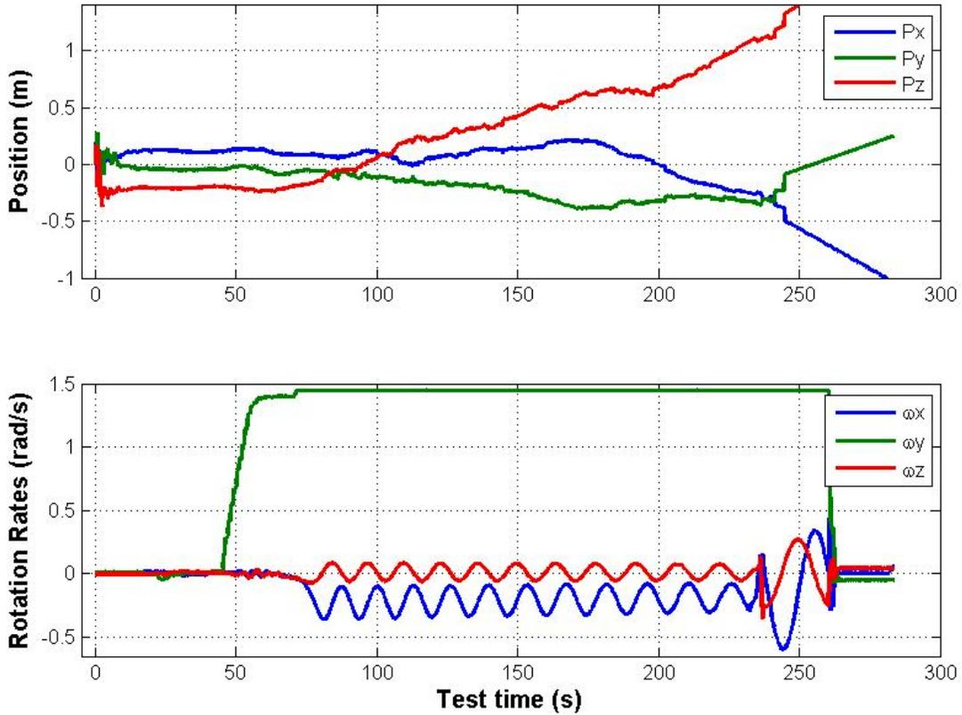
Figure 4.3 TS16 P251 T3 Fluid Slosh: SPHERE + Battery Pack, Y Rotation – Position and Rotation Rates
