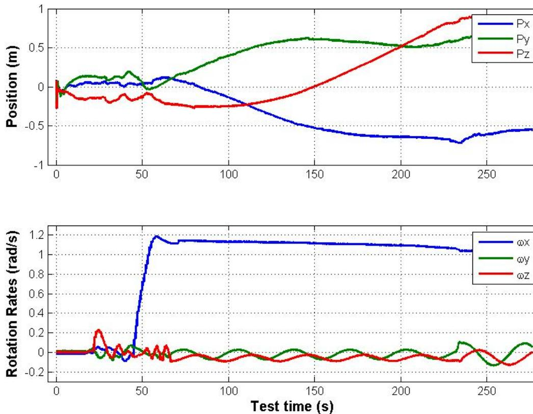
**Figure 4.1 TS16 P251 T2-3 Fluid Slosh: SPHERE Only, X Rotation – Position and Rotation Rates**
