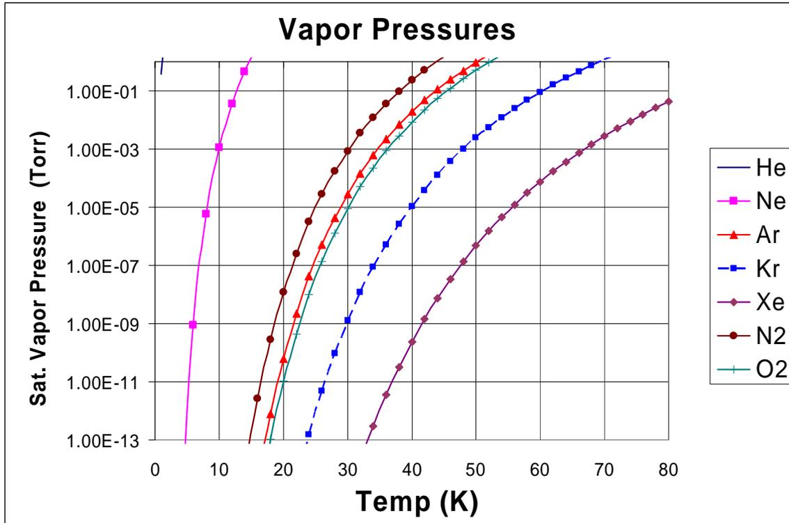
Figure 3. Saturation pressure plots using the Clausius-Clapeyron equation.
