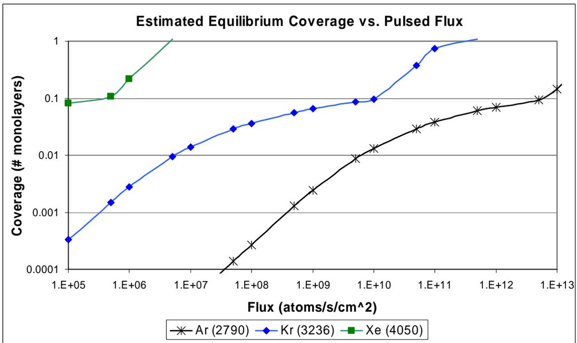
Figure 15. Equilibrium coverage for various heats of adsorption vs. pulsed flux
