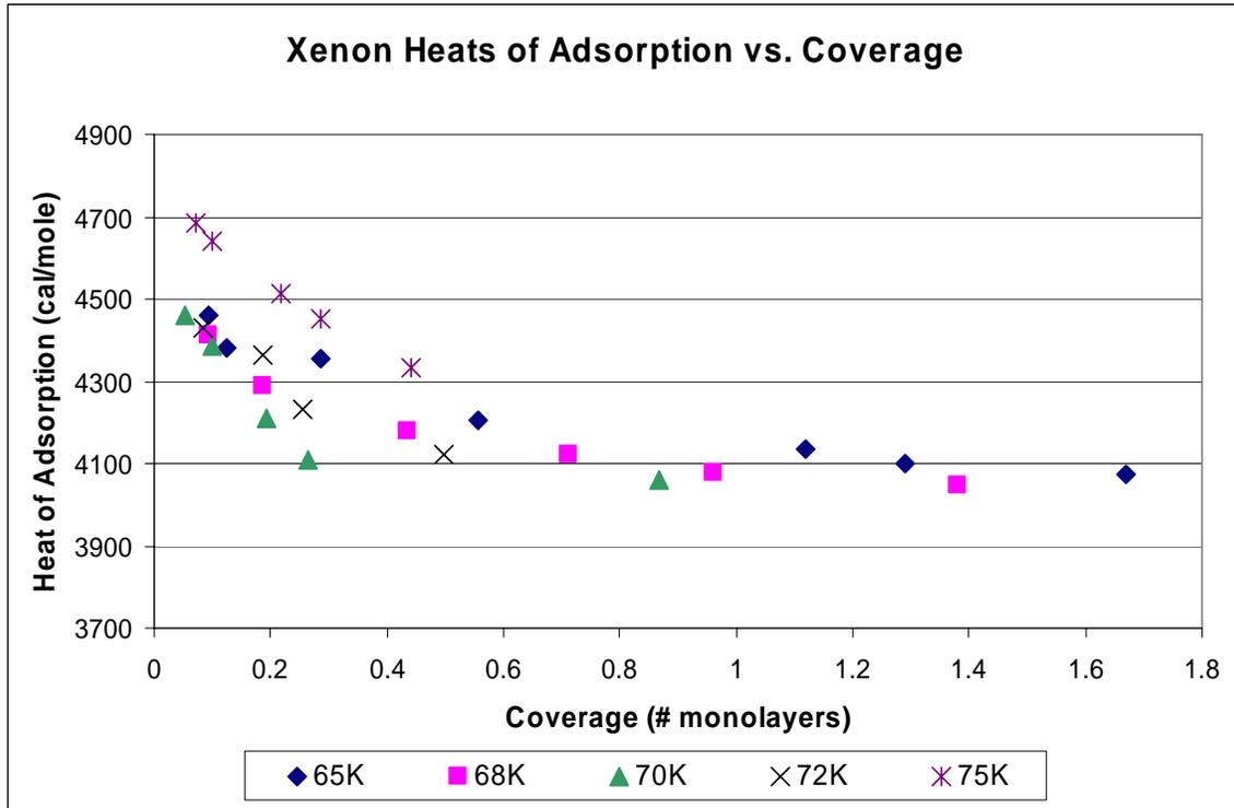
**Figure 27. Xenon heat of adsorption vs. coverage, by temperature**
