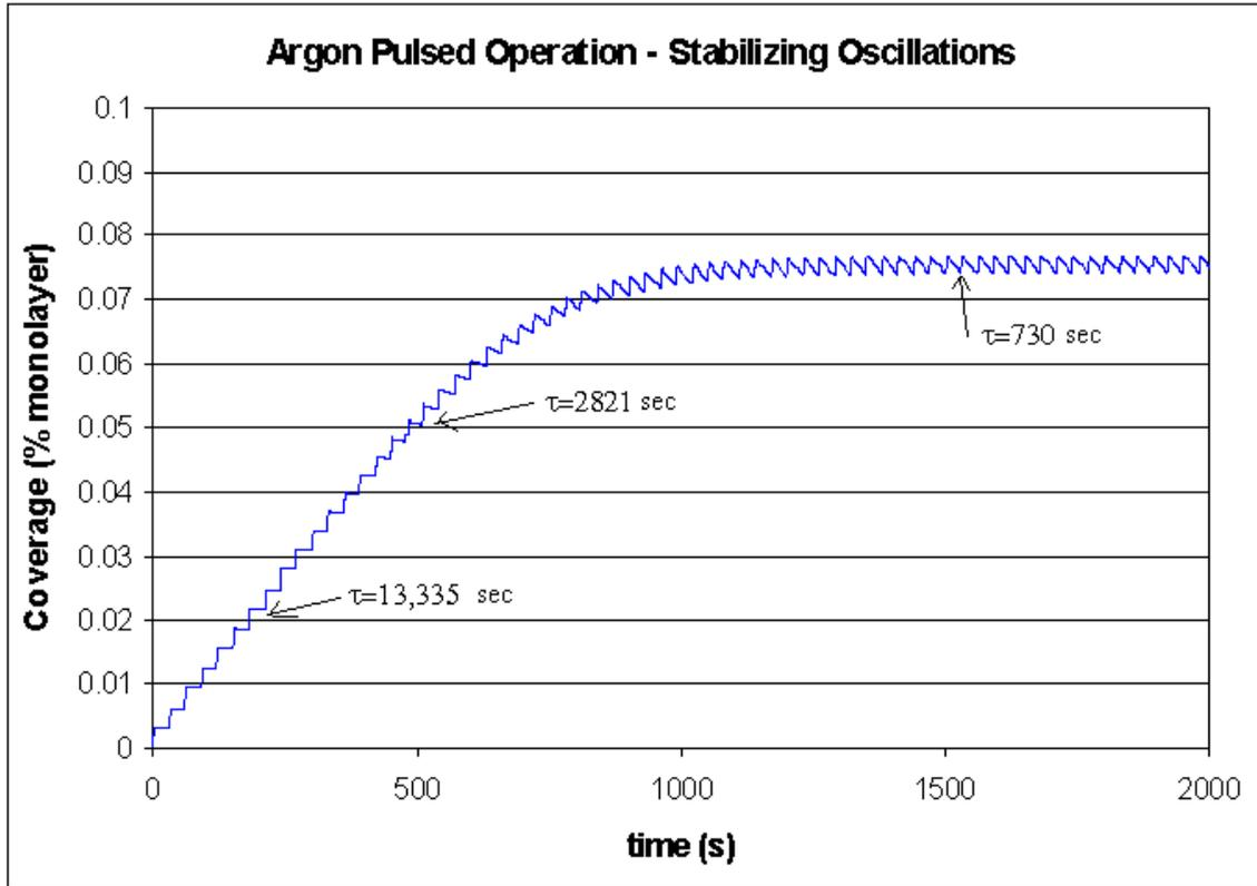
Figure 14. Equilibrium deposition behavior with pulsed thrusters
