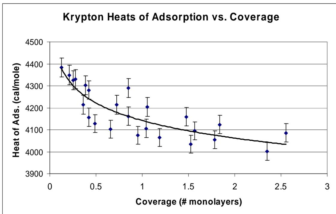
**Figure 30. Krypton heat of adsorption data with trendline**
