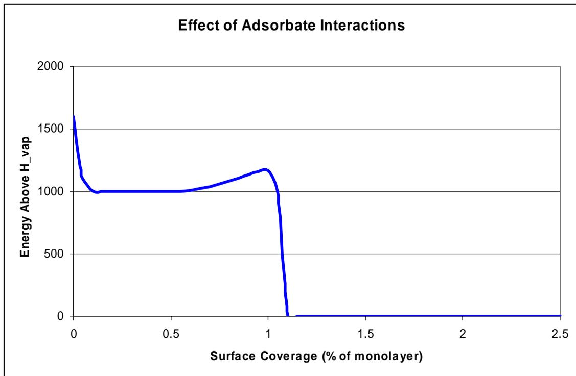
**Figure 7. Heat of adsorption with adsorbate interactions.**
