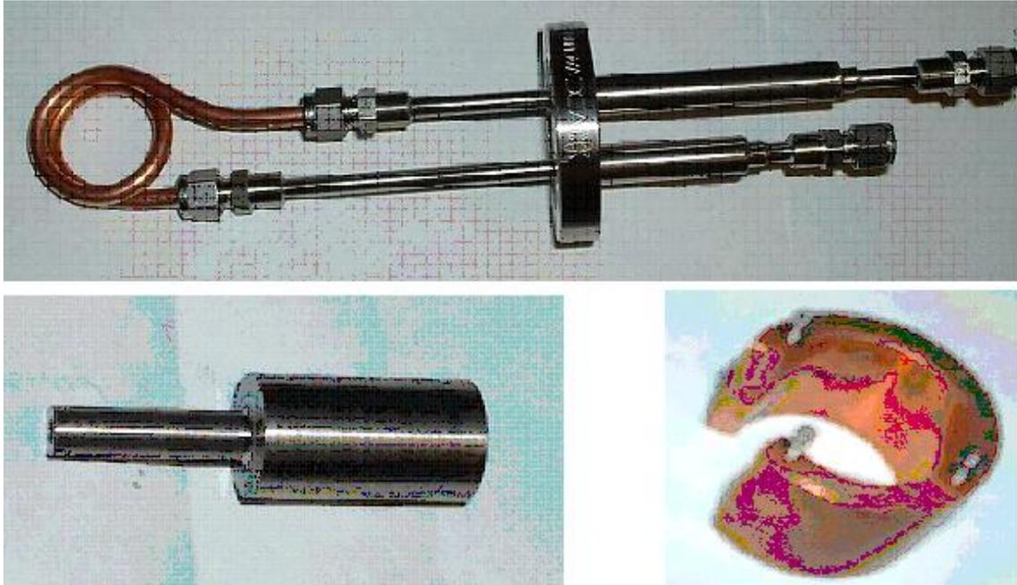
**Figure 23. Feedthrough/coil (top), adapter (left), QCM connector (right).**
