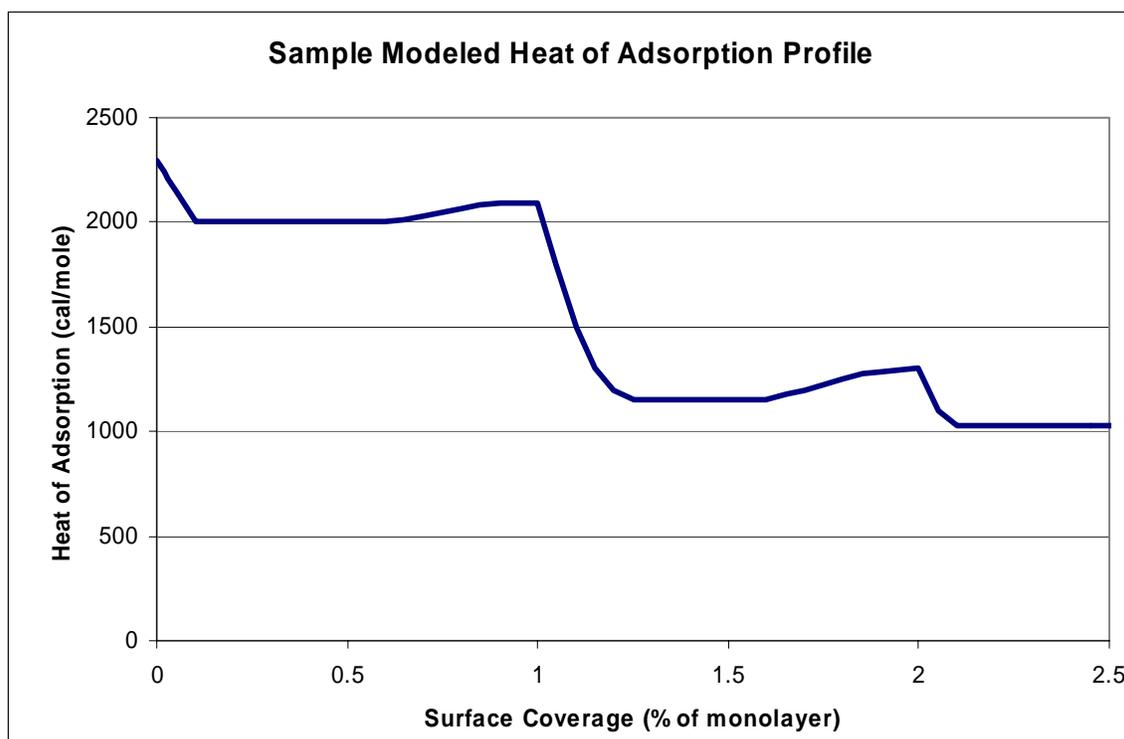
**Figure 10. Modeled heat of adsorption, surface flaws and adatom interactions.**
