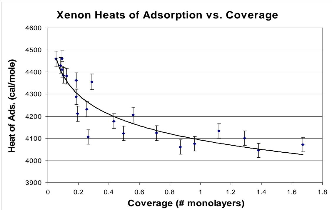
**Figure 28. Xenon heat of adsorption data with trendline**
