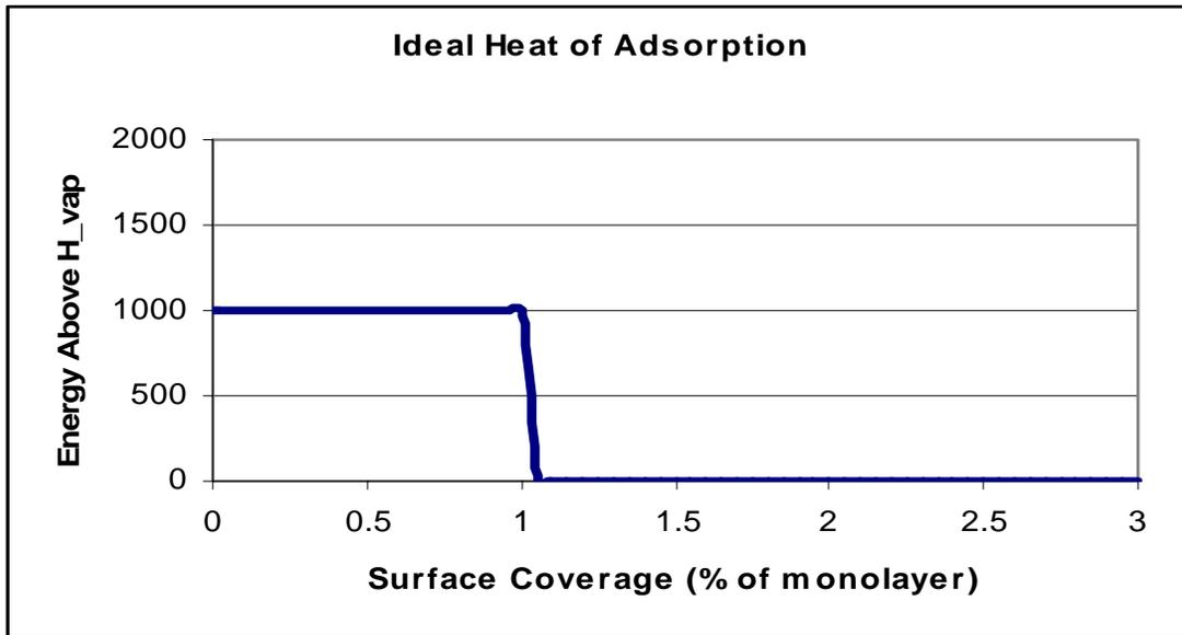
**Figure 5. Ideal heat of adsorption with perfect surface, no adsorbate interactions.**
