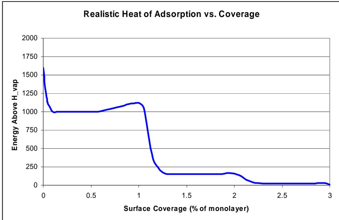
**Figure 8. Realistic heat of adsorption vs. coverage behavior.**
