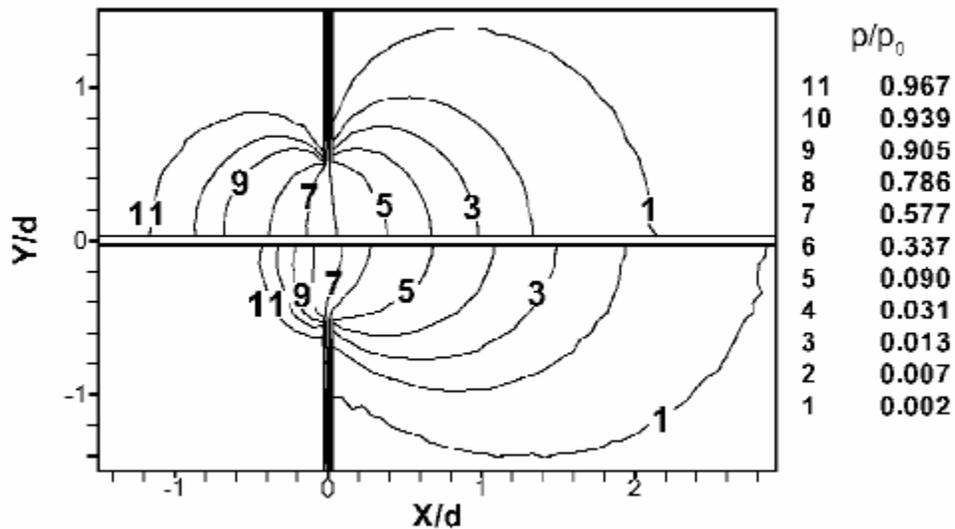
**Figure 20. Neutral flow into vacuum from an orifice.**
