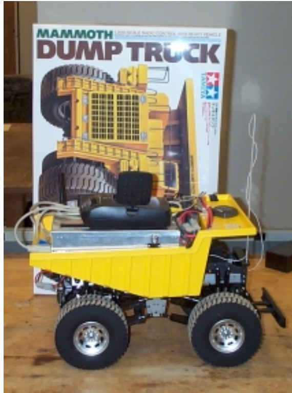
Figure 4-1: Tamiya Mammoth Dump Truck with electronics payload
