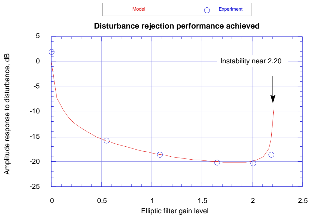
Figure 4.21 RMS attenuation of disturbance as a function of elliptic filter gain.
