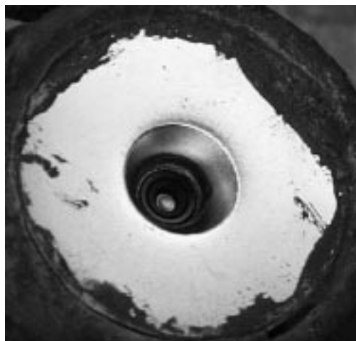
Figure 4-10: Erosion pattern at the center pole piece
