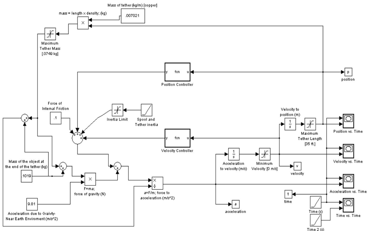
**Figure 1.** The control law for the Earth model.
