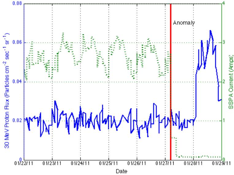
Figure 11: 30 MeV Proton Flux during SSPA Anomaly
