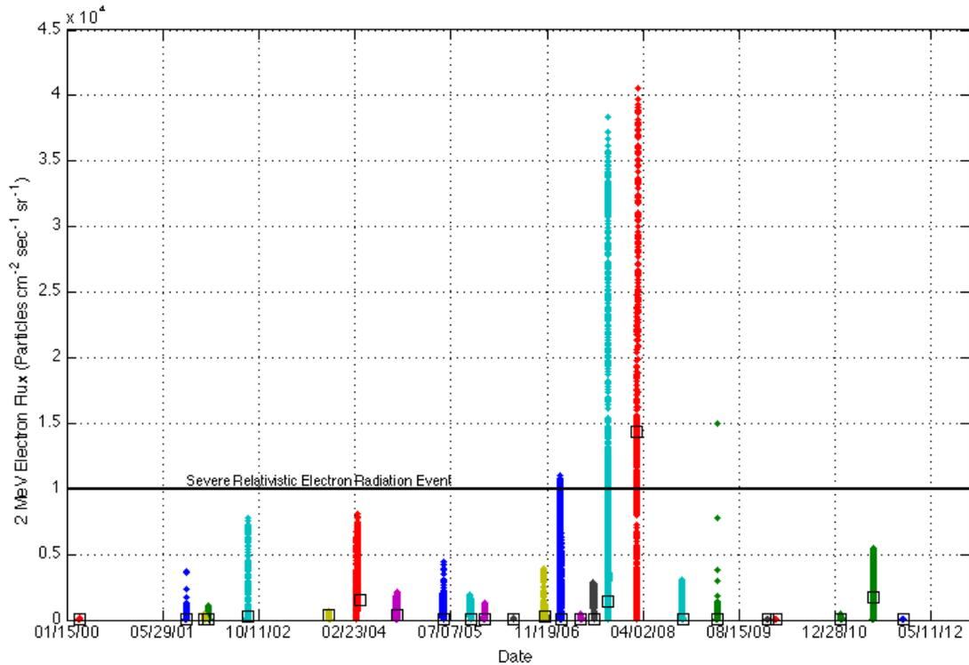
Figure 9: 2 MeV electron flux five days prior and one day after each of the SSPA anomalies, and the 2 MeV electron flux at the time of each SSPA anomaly (black squares).
