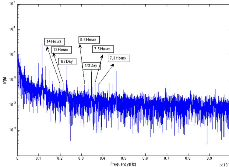
Figure 7: Single Amplitude Spectrum of Anomalous SSPA
