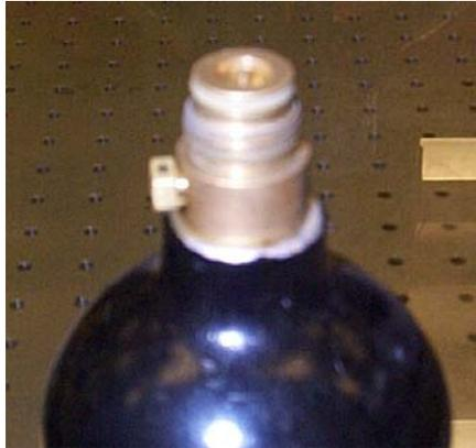
**Figure 2.8. Standard pin valve.**
